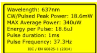
Label specifying wavelength, average power, pulse energy, and pulse length of the laser.
