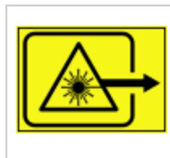
Laser aperture label. Designates the place from which laser radiation is emitted.
